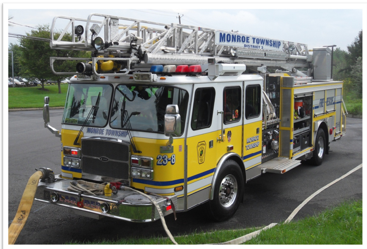
Fig 1. A Quint is a motorized fire apparatus that has a permanently mounted fire pump, an on-board water tank, an area for hose storage, an aerial/elevated platform with a permanently affixed waterway, and an ample supply of ground ladders.
